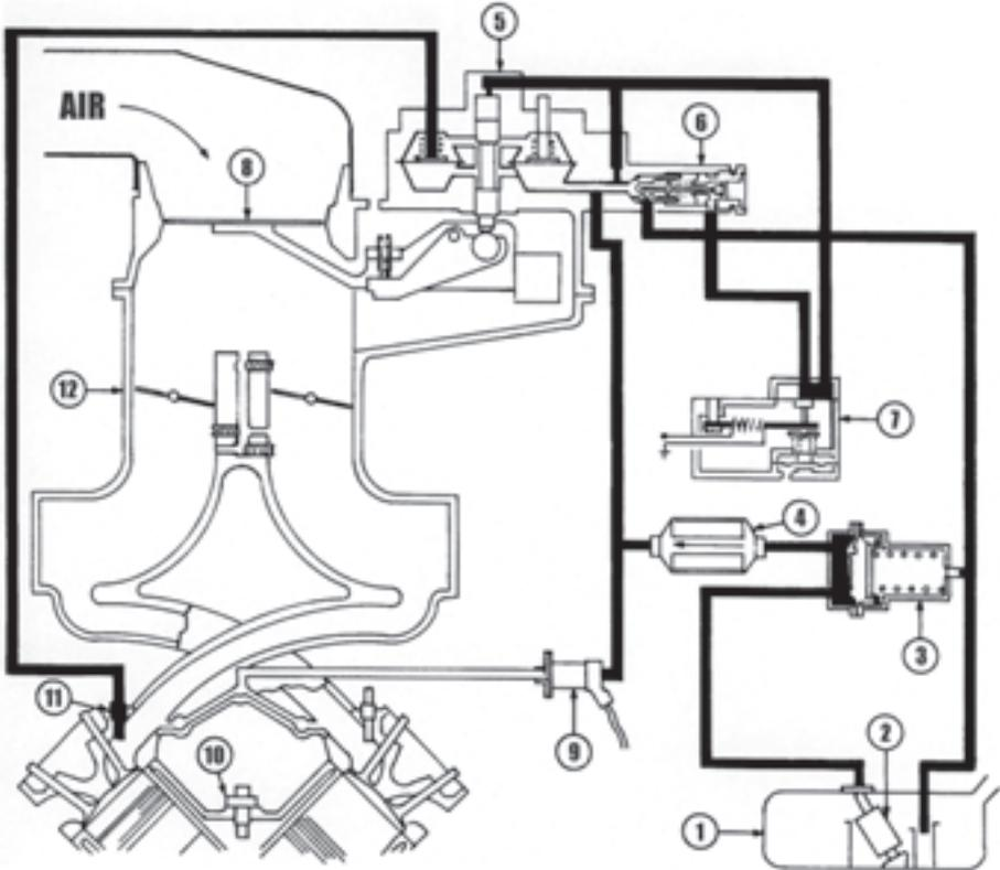
**1. Fuel Tank** - The fuel tank is blow-molded plastic, and located in the front “wishbone” of the frame. Accessing the in-tank components (*see page 88*) is most easily accomplished via the inspection cover inside the trunk, rather than by removing the tank from underneath the car.
