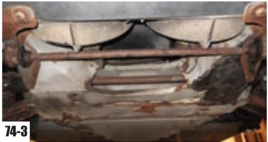
The mild steel frames were coated with a two-part epoxy with the idea that this would provide corrosion protection. In many cases, this is true, but particularly in areas where salt is used on roads, or salt air is prevalent, close attention should be noted to the condition of the frame and suspension components. The epoxy will crack with age rather than flex, and allow moisture to become trapped between the steel frame and epoxy, accelerating corrosion.
