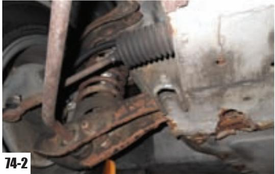
**Frame and Roof Rust:** While the stainless body, urethane bumpers and fiberglass underbody won't rust, an increasingly common problem with DeLorean cars is rust on the frame and in the roof box. Quite possibly the most expensive issue to be aware of when inspecting a DeLorean for purchase, the impact of rust on the frame, suspension components and/or roof box cannot be overstated.
